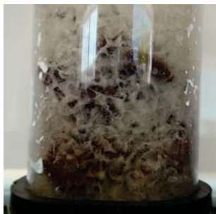
SwellLCM sealing massive voids b/w lava rock.
